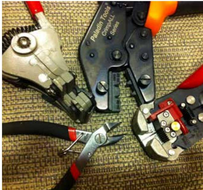
ends. ChannelLock makes some dandy cable cutting pliers (Model 911) useful for quick, clean cuts on electrical, coaxial, or multi-strand cables. I have seen them advertised for \$20-30 online, at home improvement stores, and even through Wal-Mart. Also, check the electrical tools section of your favorite hardware store.
