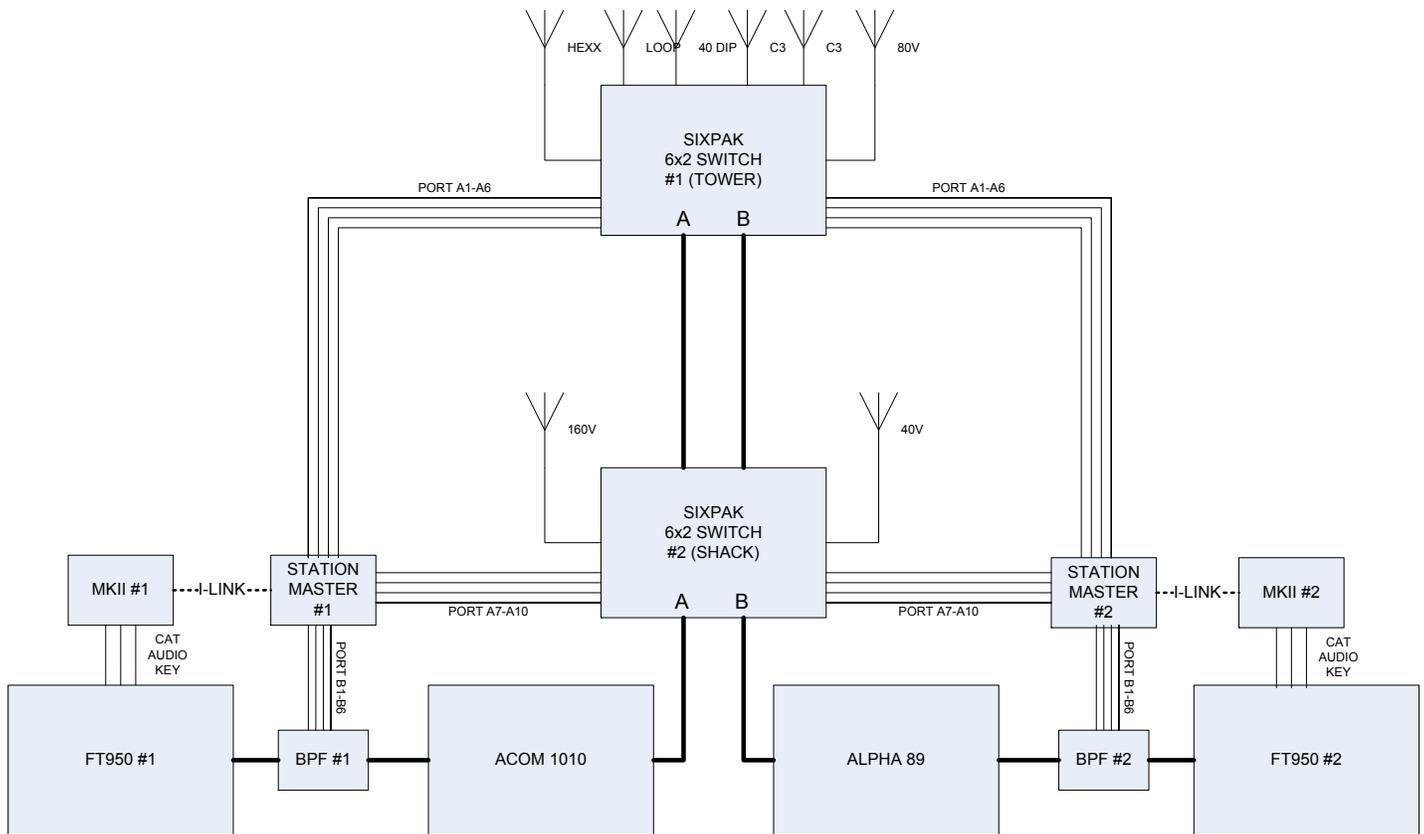
Here’s how we do two-radio operations at KL2R. Bandpass filters (BPFs) are critical to resolve any interference between the two stations running high power. The Microham Station Masters automate switching.
