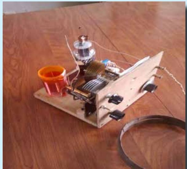
It describes a crystal set that was subsequently adapted to use a 1625 tube (12 volt version of an 807). The circuit he showed used a wall wart for 12 volt power, but I omitted that part since I want to use 12 volt battery only. My circuit is bastardized a little due to having to use what I had on hand, and uses different values for the tuned circuit, and no wall wart, series plate resistor nor the large filter cap.
