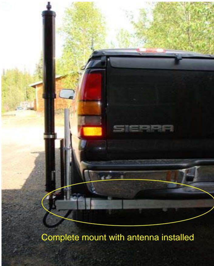
Complete mount with antenna installed
