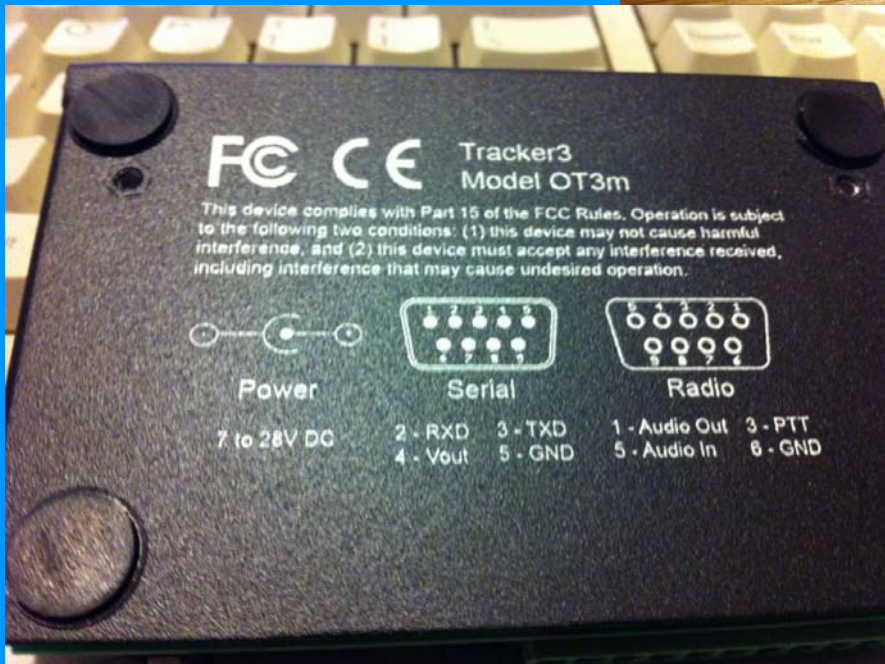
The OT3m features pin-outs silkscreened on the bottom - thoughtful in case you lose the manual.
