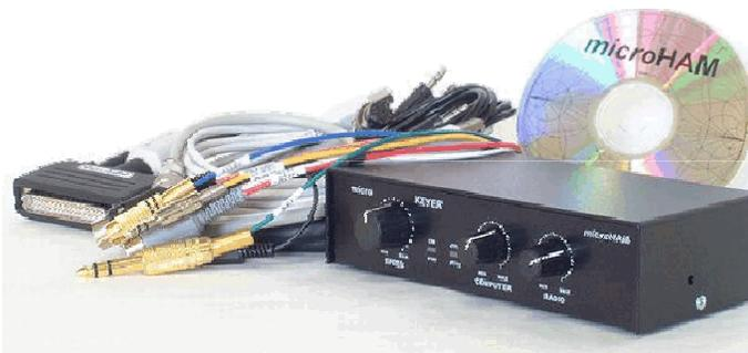
I also tried the MicroKeyer using a Windows XP laptop with 1.4 GHz Celeron M, 1 GB RAM, and AC97 integrated audio. Ham Radio Deluxe, PSK31 Deluxe, MMTTY, DXLab Suite's WinWarbler, and N1MM logger (with MMTTY integrated) all worked fairly well in CW and digital modes. The operation was fine for Field Day use. More experimentation will be required to settle on a diverse single-transmitter contest configuration.
