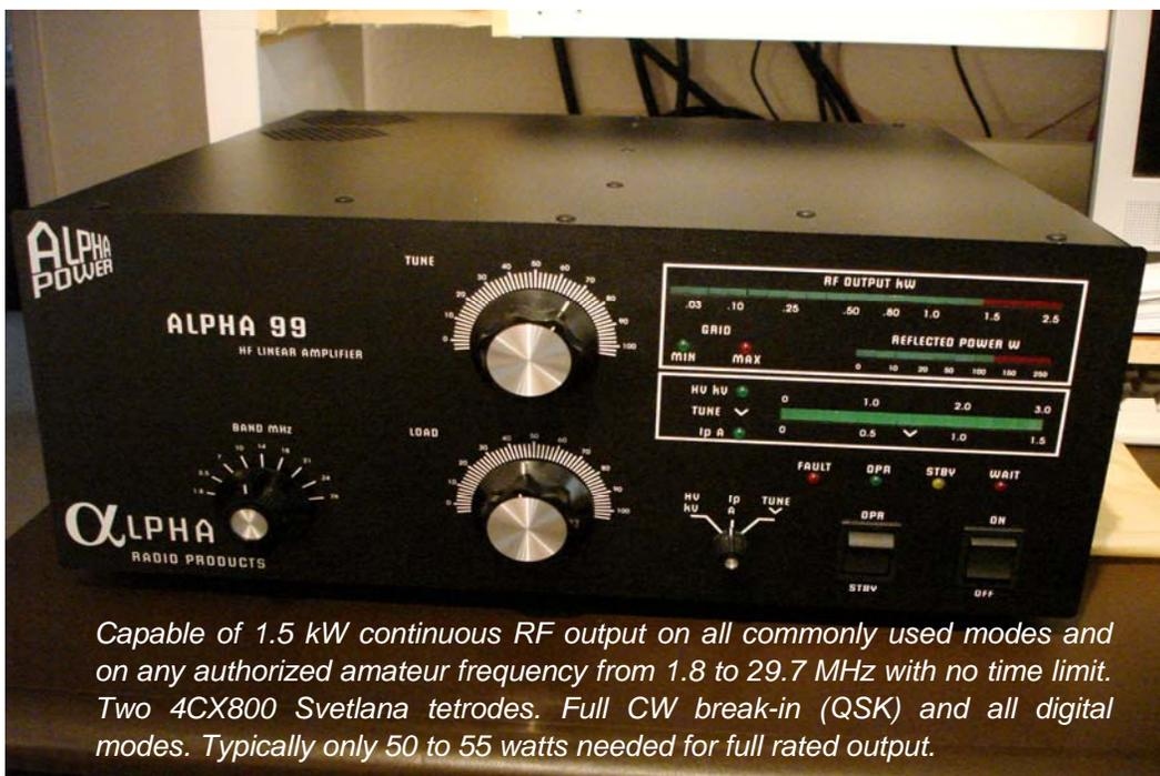
Capable of 1.5 kW continuous RF output on all commonly used modes and on any authorized amateur frequency from 1.8 to 29.7 MHz with no time limit. Two 4CX800 Svetlana tetrodes. Full CW break-in (QSK) and all digital modes. Typically only 50 to 55 watts needed for full rated output.
