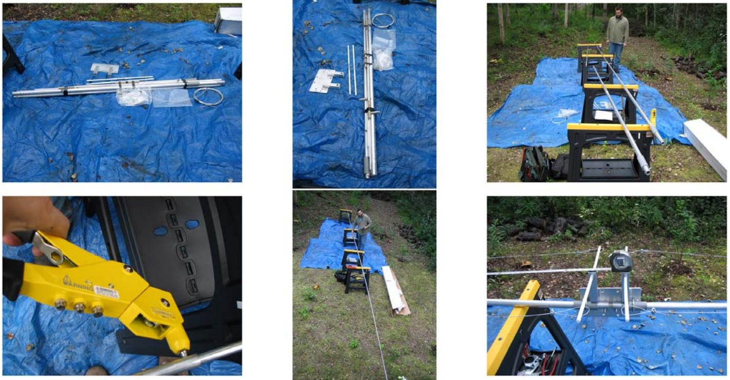
Clockwise from upper left: All EF-140 parts from the box. Note the center support plate just to the left of the pile of parts. Justin surveying side “A” and “B” main elements. The center supports/linear loading elements incorporates fiberglass standoffs and heavy aluminum wire. Fully assembled over 44 feet long. Your friend the rivet gun.
