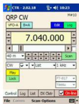
*Control your rig with a Bluetooth-enabled PDA and CTR-Remote.*
